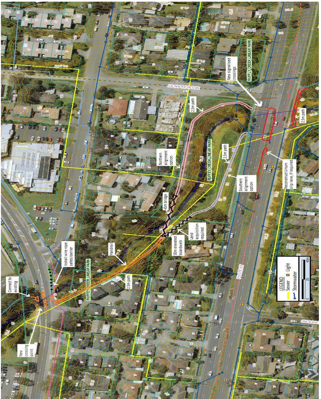
Figure 6: Proposed off-road Trail between Foote Street and Parker Street, showing route options on both sides of Ruffey Creek
